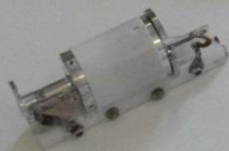
Theodore Maiman's original first laser early 1960. U.S. Patent # 3,353,115 An aluminum cylinder with flash light and ruby crystal mount. A spiral flash light and a ruby crystal with evaporated-silver-mirrored ends are enclosed in a hollow aluminum cylinder.
